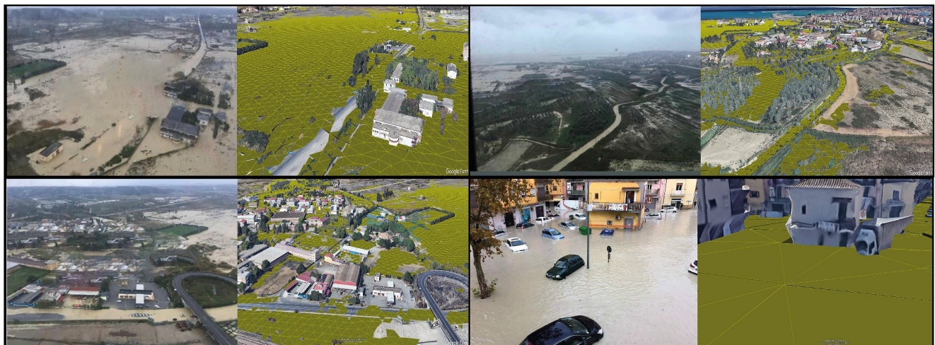
Figure 9. 3-D graphical comparison between real flooding photographs and simulated flood extent (maximum envelope of the depths from 20 November 2020 00:00 to 22 November 2020 00:00).
