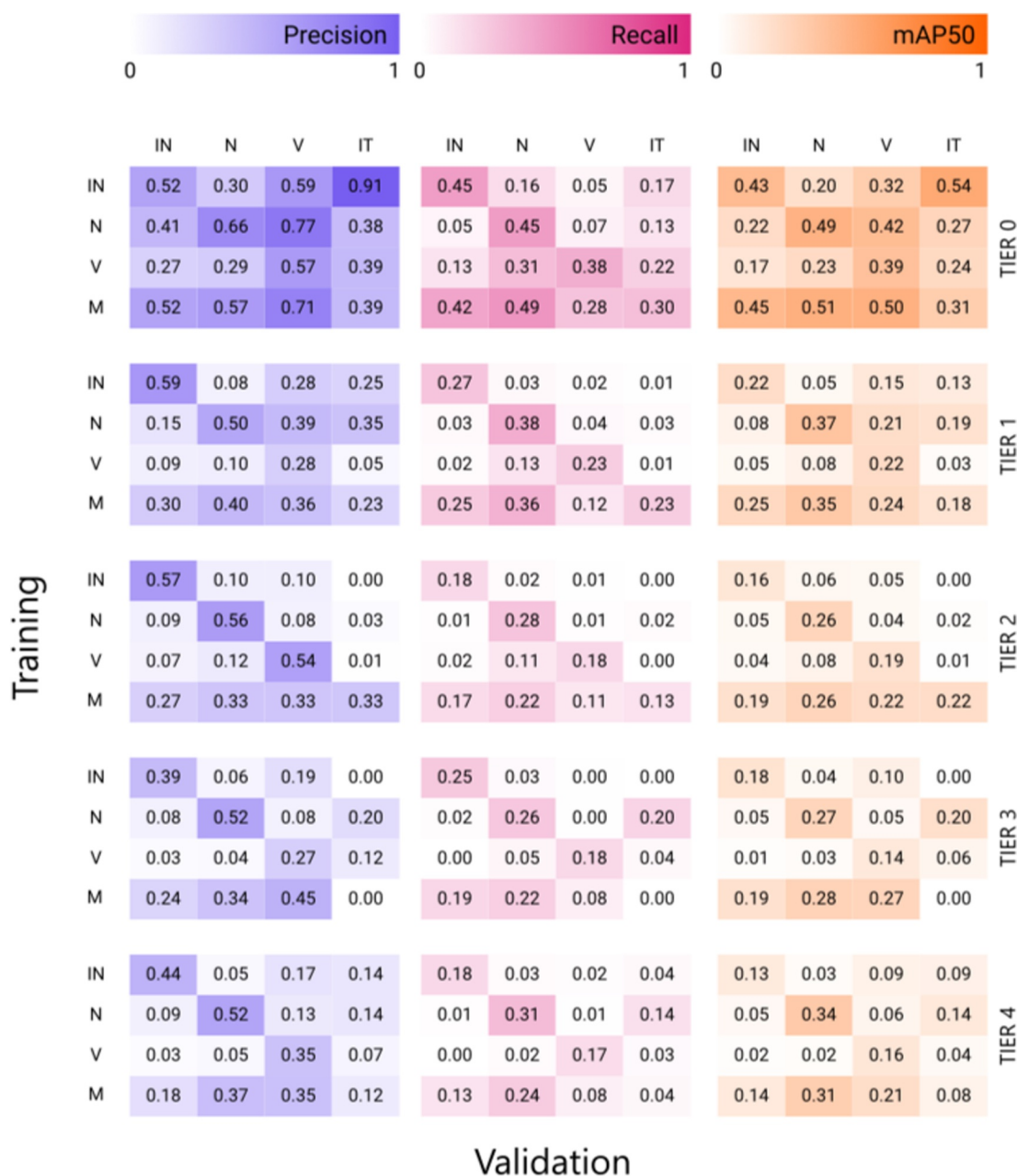
Figure 9. Model Transferability using YOLOv8 for overall model performance with external data set (IT-Italy) and other training data sets. Note that all single site data sets (IN-Indonesia, N-The Netherlands, and V-Vietnam) are included in the model training of the Mixed (M) data set.
