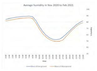
**Figure 5:** Average humidity on the soil surface from the IoT sensors installed on the eastside and the westside of the ancient sandstone Buddha
