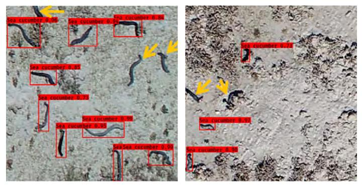
**Figure 1.** Detection result from a preliminary deep learning object detection model. The red boxes show the location of each sea cucumber. The number on top is the confidence score generated by the detector automatically showing the certainty of the results (from 0 to 1, i.e., from not confident to very confident). The yellow arrows are the sea cucumbers that the detector missed.
