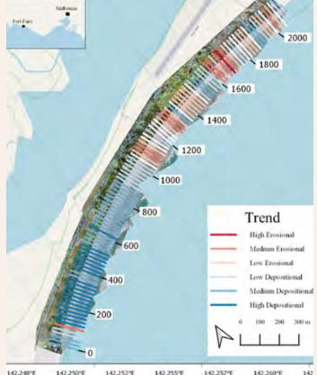
**Figure 3:** Transect-level behavioural regime (r-BCD index, see full paper for more info) in Port Fairy East Beach derived from three-dimensional change timeseries of sand-only points, highlighting the expected erosional hotspots at the end (up-drift) of the rockwall.
